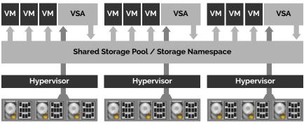
Figure 1-1: An overview of a Virtual Storage Appliance
