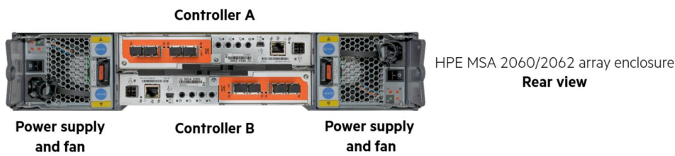
FIGURE 3. Rear view of an HPE MSA 2060/2062 array enclosure
